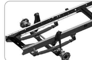
Front Parabolic Suspension and Rear Semi-elliptical Suspension
