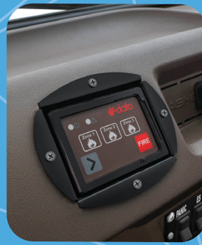
Fire Detection & Alarm System*
